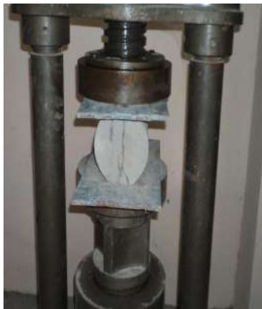
Fig 3 : Split tensile test on concrete
