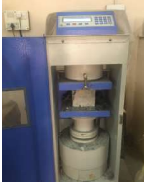
Fig 2. : Compression test on concrete
